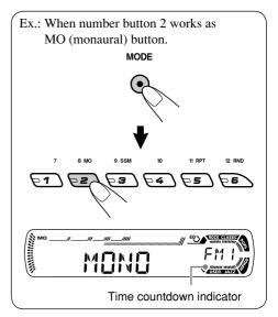
To use these buttons for original functions again after pressing MODE, wait for 5 seconds without pressing any of these buttons until the functions mode is cleared.
